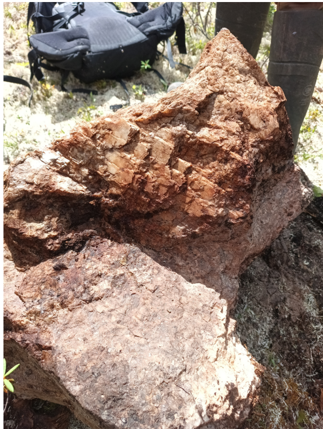
Photo 4: Sample G353065 : 4.74% Li 2 O - Angular metric boulder of spodumene-bearing pegmatite. UTM18 674,486 mN 5,907,802 mN.
