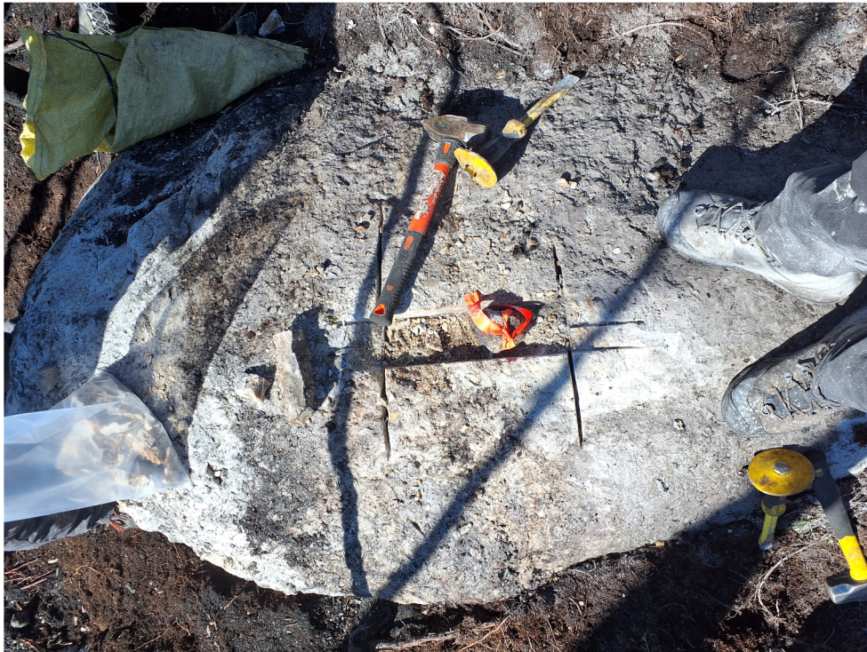
Photo 2: Sample G353039 : 1.93% Li 2 O - Subrounded metric boulder of spodumene-bearing pegmatite. UTM18 658,946 mE 5,899,873 mN.
