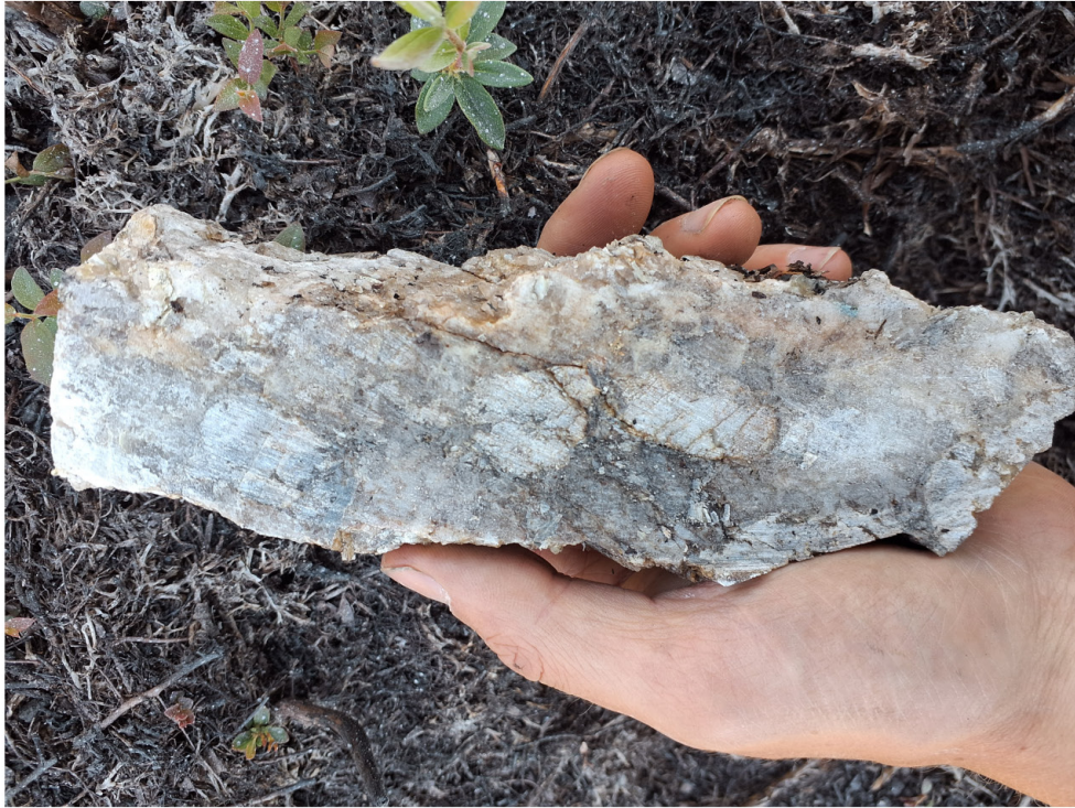
Photo 1: Sample G353039 : 1.93% Li 2 O - Sawed sample of a subrounded metric boulder of spodumene-bearing pegmatite. UTM18 658,946 mE 5,899,873 mN.
