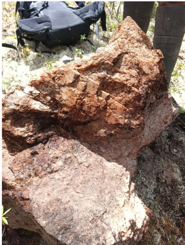
Photo 4: Sample G353065 : 4.74% \text{Li}_2\text{O} - Angular metric boulder of spodumene-bearing pegmatite. UTM18 674,486 mN 5,907,802 mN.
