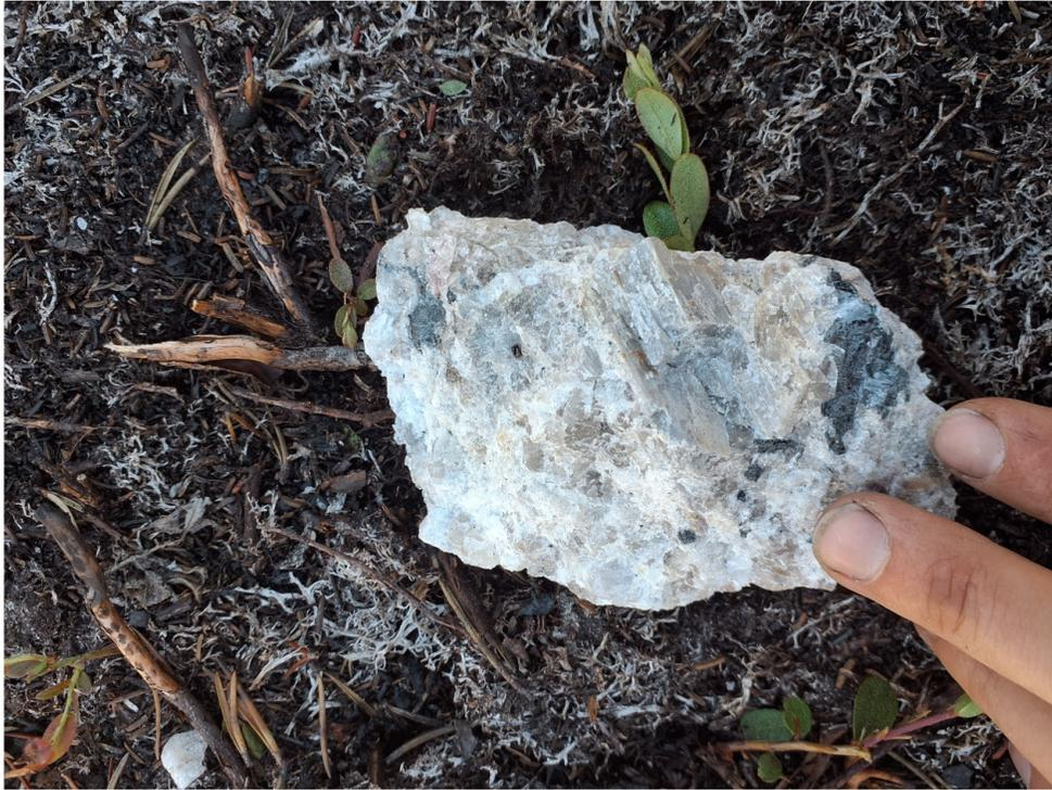
**Photo 3:** Sample G353040 : 2.85%  $\text{Li}_2\text{O}$  - Boulder of spodumene-bearing pegmatite. UTM18 659,635 mE 5,900,128 mN.
