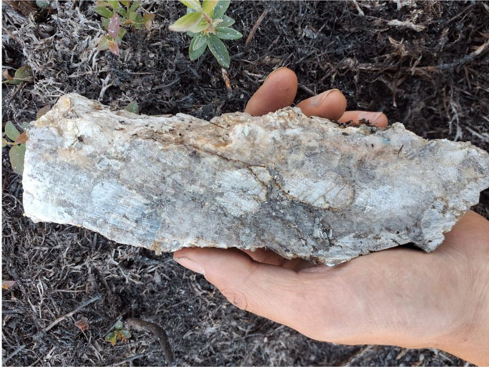
**Photo 1:** Sample G353039 : 1.93%  $\text{Li}_2\text{O}$  - Sawed sample of a subrounded metric boulder of spodumene-bearing pegmatite. UTM18 658,946 mE 5,899,873 mN.
