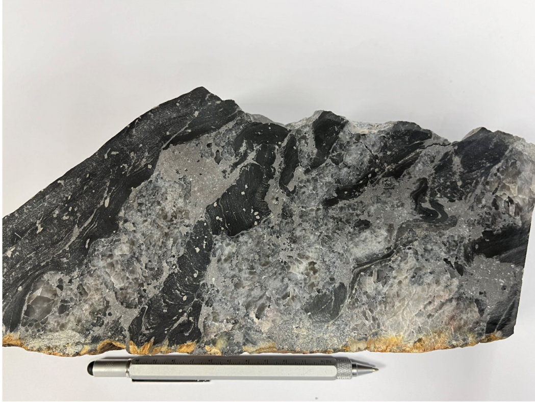
Photo 5 - Semi-massive stibnite mineralization in quartz veins with folded metasedimentary fragments. 18.15% Sb (sample E6320453).
