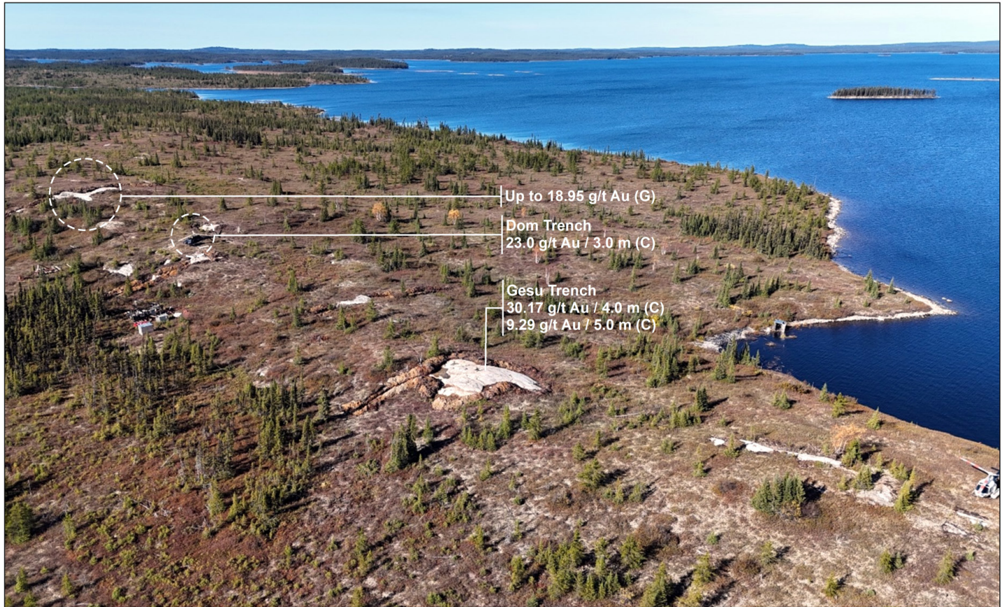
Photo 1 - Rosa Zone – General view looking north-west and selected results (C: channel; G: grab)
