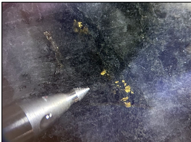
Photo 5 - Hole WR26-44 at 136.45 m. Native gold grains in quartz veinlets with biotite, tourmaline, chlorite, and traces of arsenopyrite, pyrrhotite, chalcopyrite. Sample 24366464 : 5.15 g/t Au / 1.5 m (from 136.0 m).
