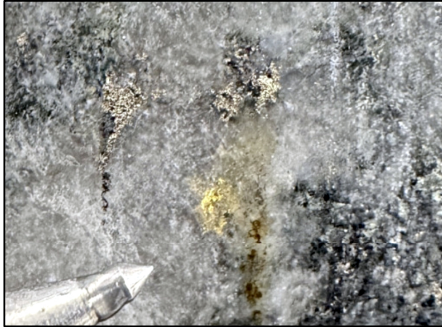
Photo 1 - Hole WR26-30 at 136.7 m. Native gold grains in quartz-chlorite ± carbonate veinlets with pyrrhotite, chalcopyrite in silicified metasediments. Sample 2435119: 2.72 g/t Au / 1.0 m (from 136.0 m).
