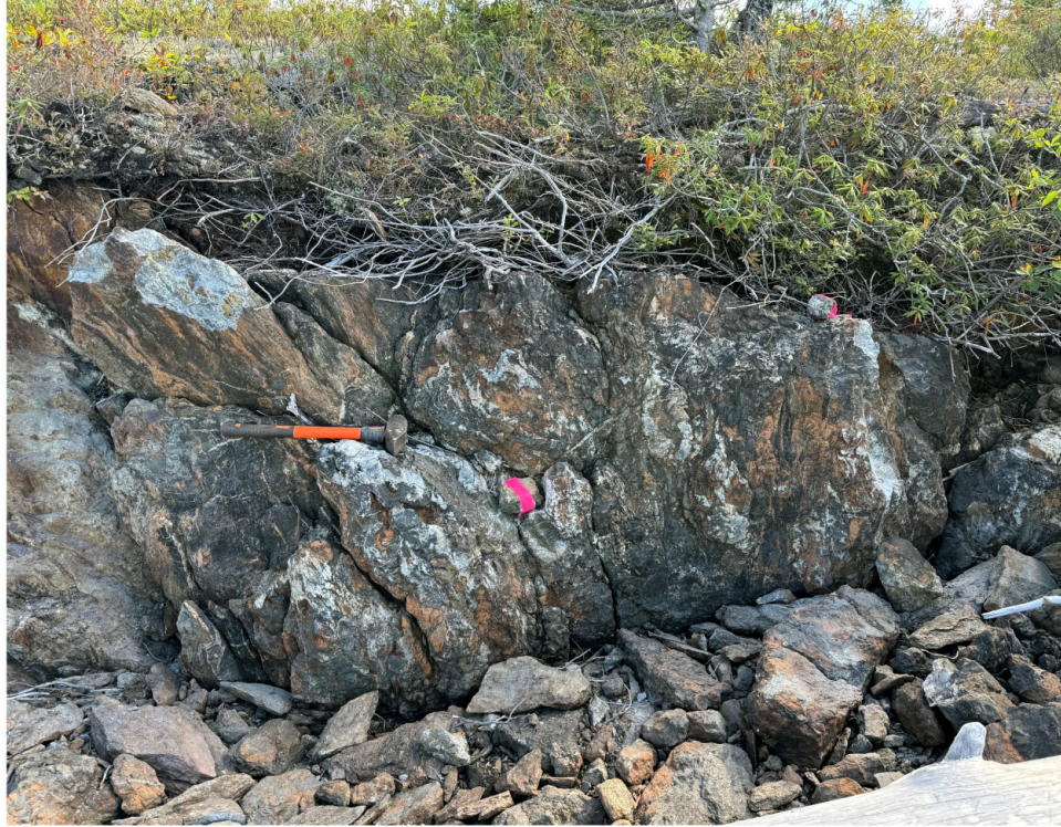
Photo 1 - Strongly mineralized outcrop with semi-massive to massive arsenopyrite (>30%), pyrite, chalcopyrite, quartz-iron carbonate veinlets, tourmaline and sericite.
